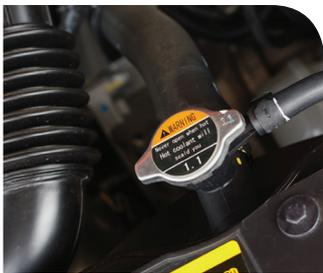
The cooling system in your car is one of the most important systems to keep well maintained. Antifreeze prevents freezing, raises the boiling point and prevents corrosion of internal components. Most vehicle manufacturers recommend a two-year service interval.
