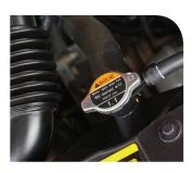
The cooling system in your car is one of the most important systems to keep well maintained. Antifreeze prevents freezing, raises the boiling point and prevents corrosion of internal components.
